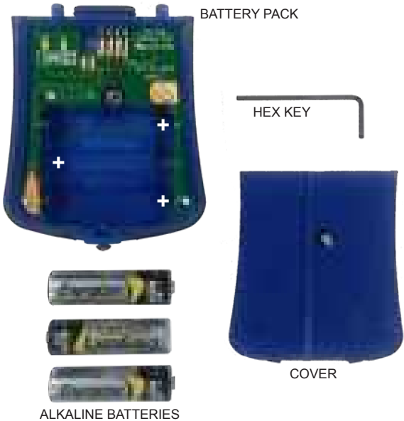
Fig. 4.13 Alkaline Batteries Removed
