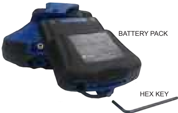
Fig. 4.11 Battery Pack Removed
