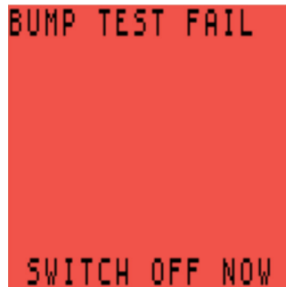
Figure 6-8: Bump Test Fail - Switch Monitor OFF
